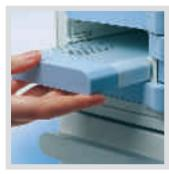
Plug-in battery modules are powerful for their size and weight, adding to convenience during the process of transporting the patient
